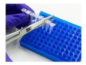
**3.** Transfer 5  $\mu$ L of positive control solution into the tube containing PD1 diluent from step 8 of the XRT test kit user guide and **mix well.**
