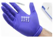
Reaction Pellets are light sensitive. Immediately place remaining reaction pellets back into the desiccated tube and then insert the desiccant tube into the foil pouch to protect from light. **5.** Transfer  $25 \mu$  from the colored tube containing your sample extract into the reaction pellet (clear tube).
