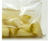
**4.** Secure the bag on an orbital shaker and shake overnight at 60 to 90 rpm (enough so that water moves freely around all tuber cores) at room temperature.
