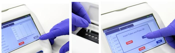
**7.** After 20 minutes of total run time the instrument will beep, indicating the test is complete. The test results will be visible next to the well designation on the screen, and should be interpreted as follows:
