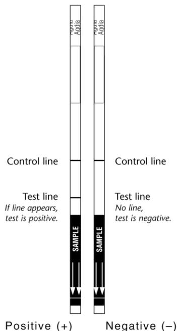
The control line can appear in as little as 3 to 5 minutes. Maximum reaction occurs in 30 minutes at which time the ImmunoStrip should be removed from the buffer. The control line assures that the test is working properly. If the control line does not appear, the test is invalid.
