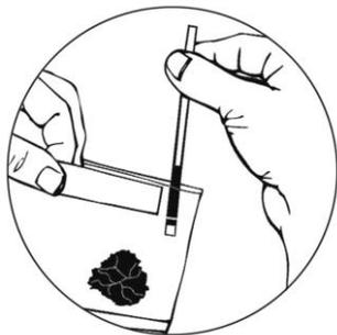
Samples can be tested directly in the bag.
