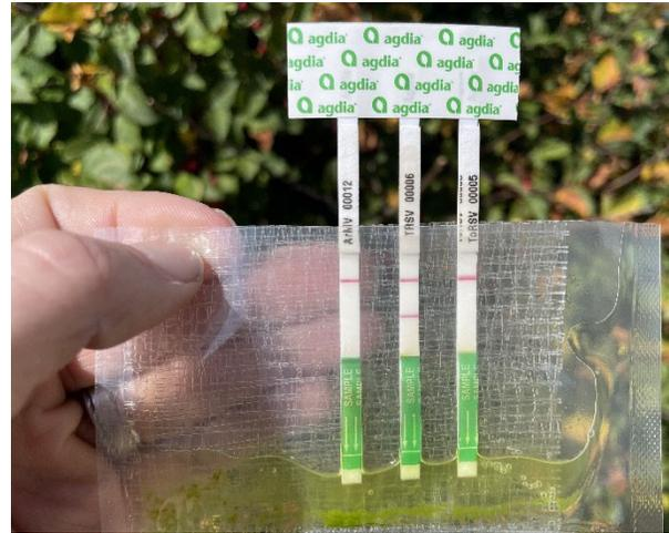
**Figure 1.** The new Nematode Viruses ImmunoComb® for convenient detection of ArMV, TRSV & ToRSV, showing results for a TRSV-positive sample.
