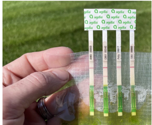
Figure 1. The new Aphid Mosaic Viruses ImmunoComb® for convenient detection of AMV, CMV, Potyviruses & TAV, showing results for a CMV-positive sample.
